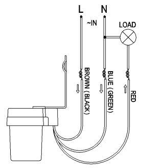
light of the controlled area and, depending on the light, the sensor turns on/off the load automatically. The ambient temperature and humidity cannot affect the proper work of the sensor. This sensor is appropriate for automation of street and garden lighting, which works only at night.
